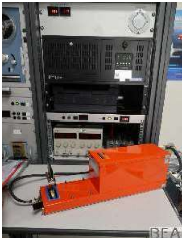
Figure 13: readout of the memory board on BEA HFR5-D chassis
