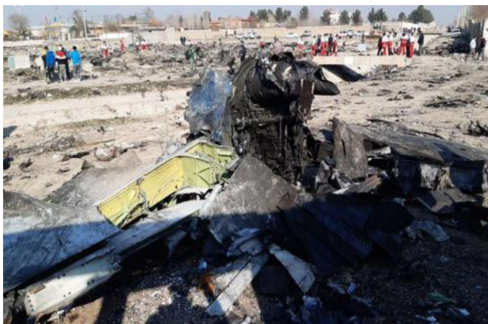
Figure 13- Auxiliary Power Unit
