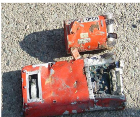
Figure 36- CVR physical appearance after the crash
