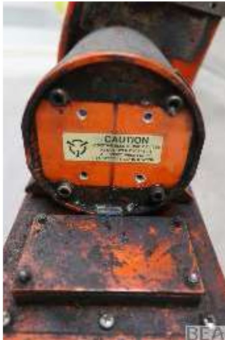
Figure 8: beacon separated from the FDR CSMU
