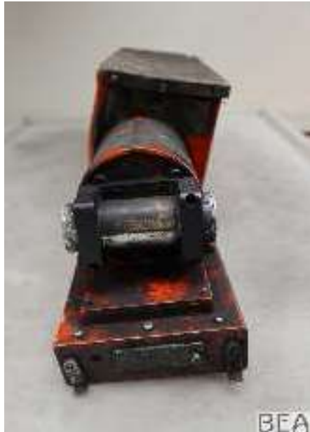
Figure 7: FDR chassis and CSMU
