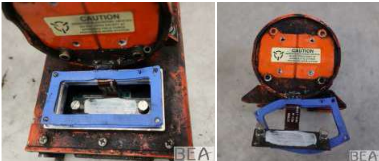
Figure 9: Separation of the FDR CSMU from the chassis
