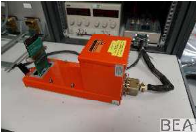
Figure 6: readout of the memory board on BEA HFR5-V chassis
