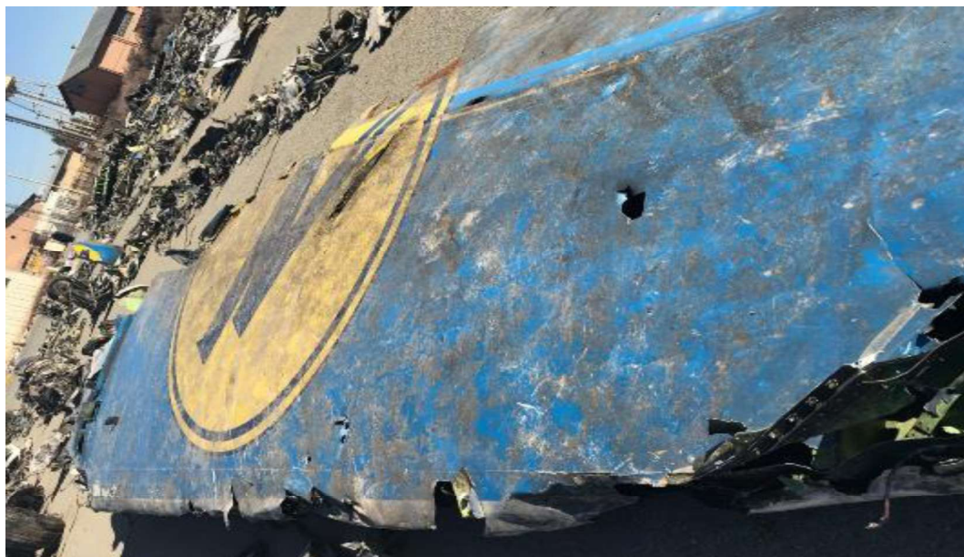
Figure 21- Holes and cracks on vertical stabilizer
