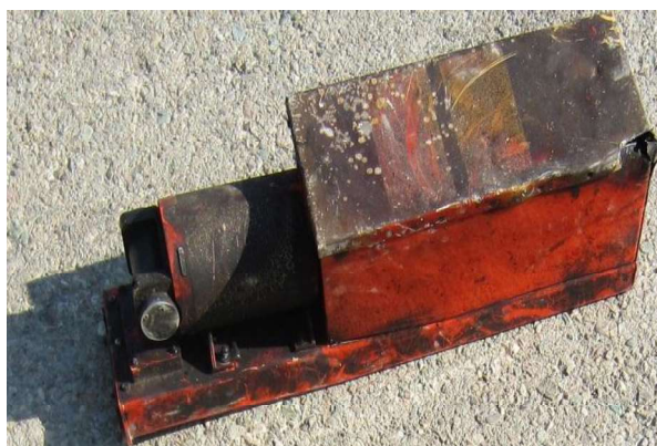
Figure 35- FDR physical appearance after the crash
