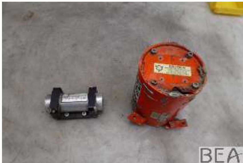
Figure 2: Beacon separated from the CSMU
