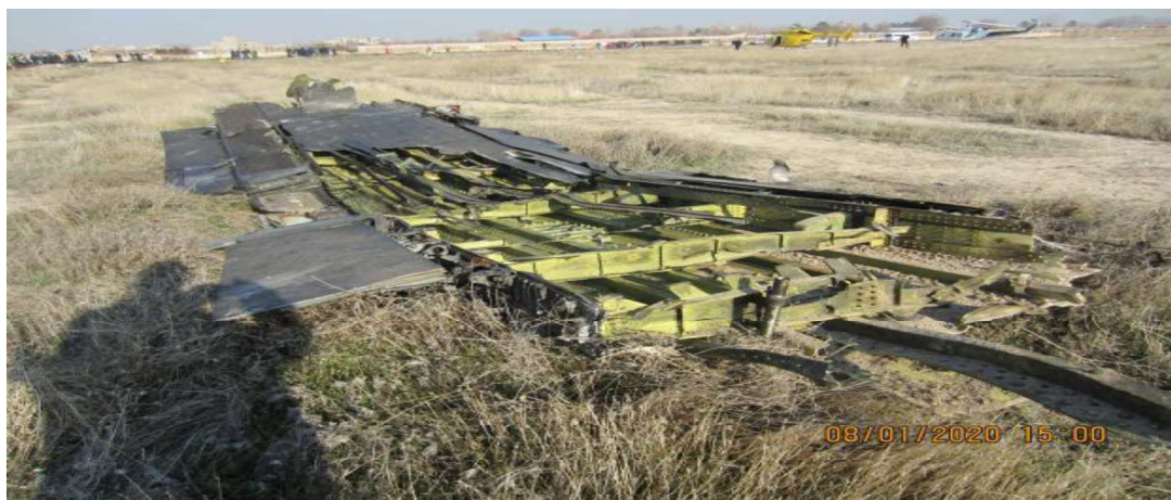
Figure 11- The aircraft left wing at the crash site
