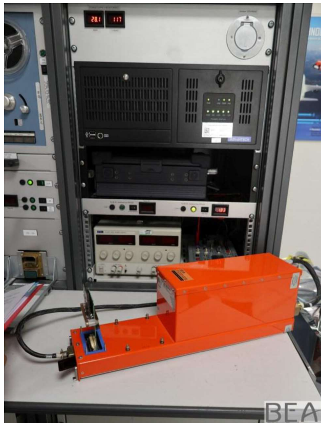
Figure 39- FDR memory card read-out at BEA laboratory using donor-chassis - Photo: BEA
