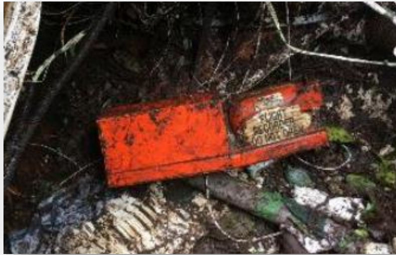
Figure 12. Condition of FDR upon recovery
