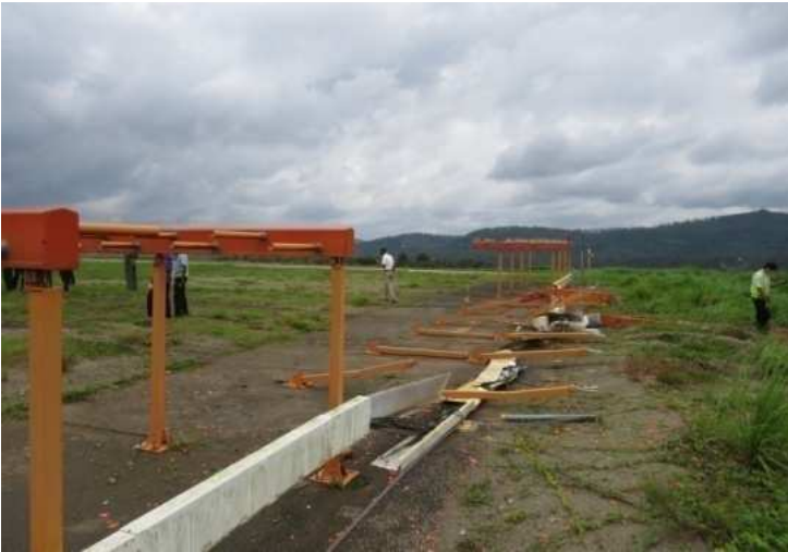
Figure 4: Damage to ILS Localiser Antenna
