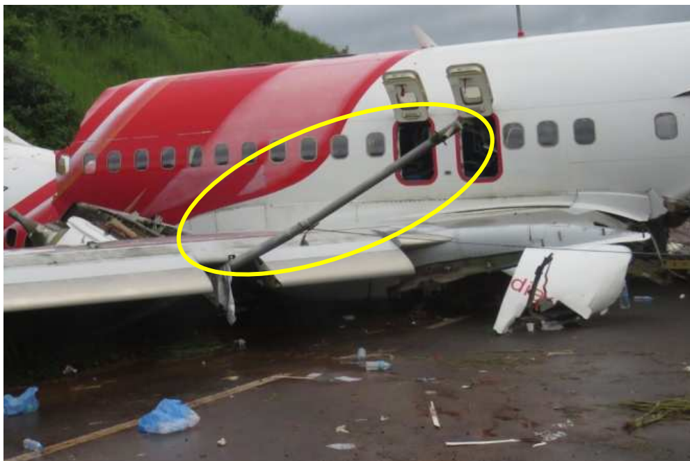
Figure 6: Lamp post broken by impact with right wing
