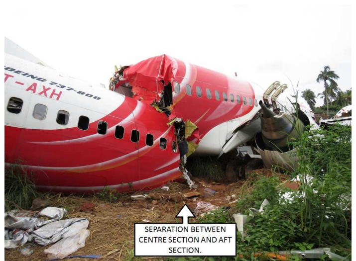
Figure 35: Separation Between Centre and Aft Section
