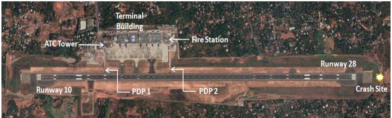
Figure 14: Aerodrome Layout (PDP: Pre Determined Point for CFT during Aerodrome Warning)
