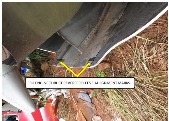
Figure 38: Engine Thrust Reverser Sleeve Alignment Marks
