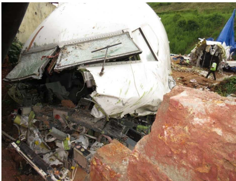
Figure 44: Front View of the Damaged Nose Section.
