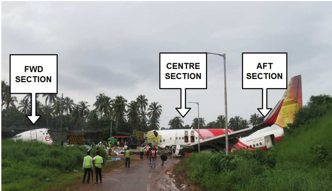
Figure 2: Aircraft broken into three sections.
