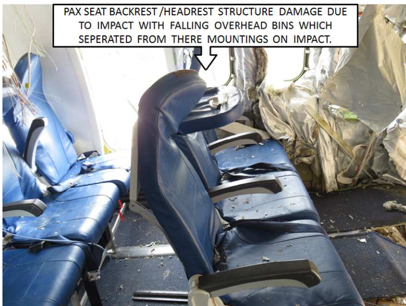
Figure 30: Passenger Seats with damaged Headrests
