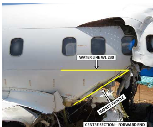
Figure 31: Centre section impact profile
