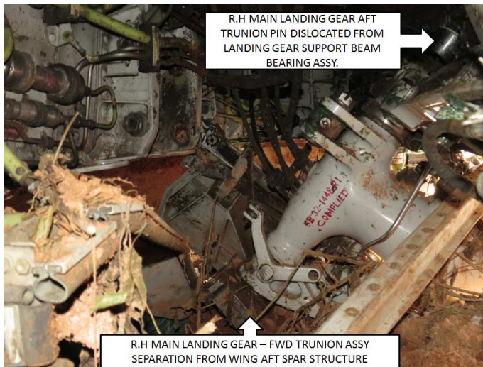
Figure 40: Right Main Landing Gear Separation
