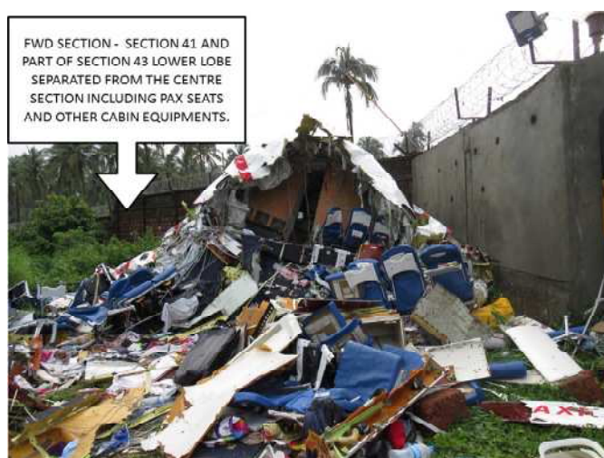
Figure 29: Forward Section Debris
