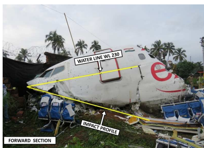
Figure 28: Forward Section Impact Profile.
