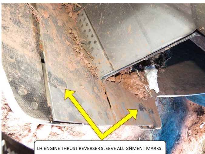
Figure 38: Engine Thrust Reverser Sleeve Alignment Marks
