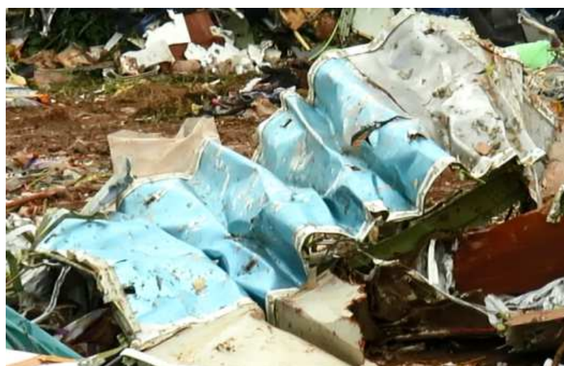
Figure 32: Centre Section Debris
