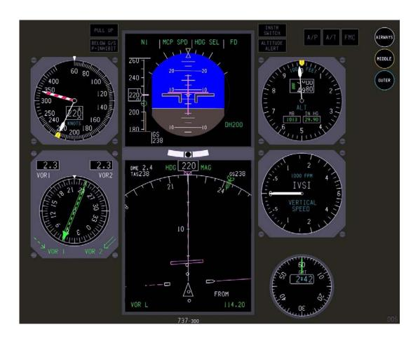
Figure 1.6.2-1 Example Captain's Instrument Display
