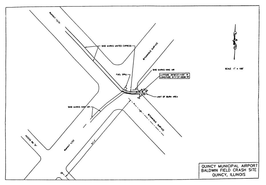
Figure 1.—Diagram of accident site.
