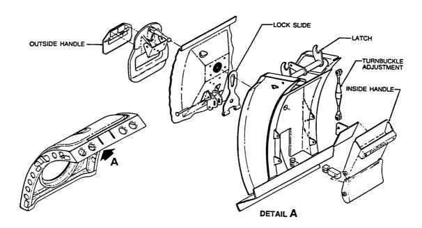
Figure 5.—Diagram of overwing exit hatch.
