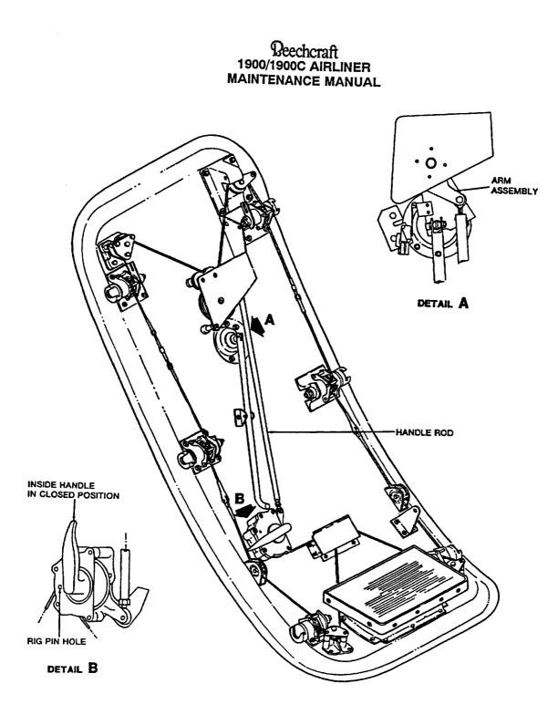
Figure 4.—Beech 1900/1900C air stair door and latching mechanism.
