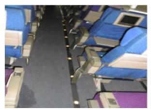
Figure 1.3-1 Illuminated Floor Proximity Lights during Testing
