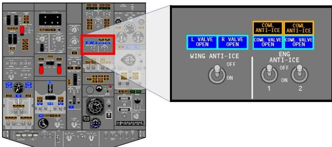
Figure 4. Location of Engine Anti-Ice Switches on the Overhead Panel P5 (Image Copyright © Boeing. Reproduced with permission, modified)
