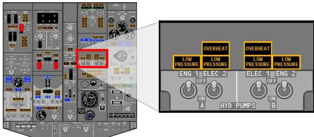
Figure 3. Location of hydraulic pump select switches on the Overhead Panel P5 (Image Copyright © Boeing. Reproduced with permission, modified)
